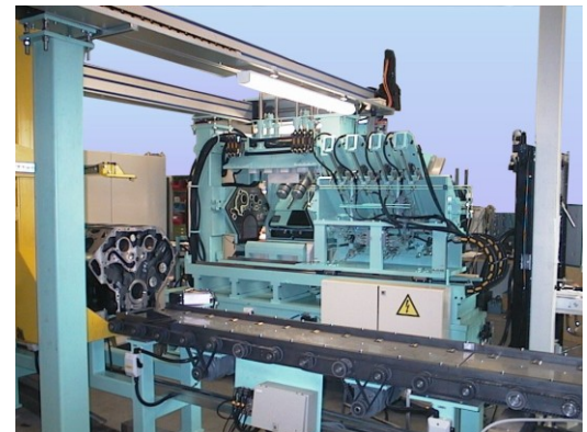
Cast Iron - fully machined V8 cylinder block - automatic linear transfer
